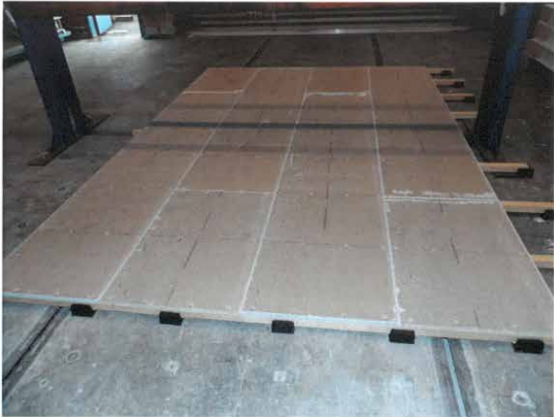
Photograph 2. Specimen ready for test
